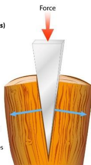
A downward force produces forces perpendicular to its inclined surfaces
